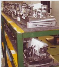
Prepared GPS 240 pallets ready for rapid introduction into the high-speed milling machines.
