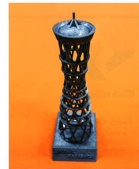
Source: Ifuku Seimitsu Co., Ltd. A finished sample of the 'Kobe Port Tower' made using a metal 3D printer
